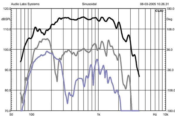
Figure 30: **Standard** 500-type, response and distortion
