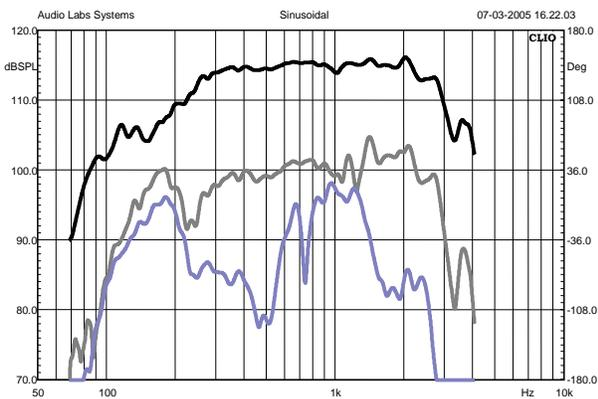
Figure 38: **Standard** 600-type, response and distortion
