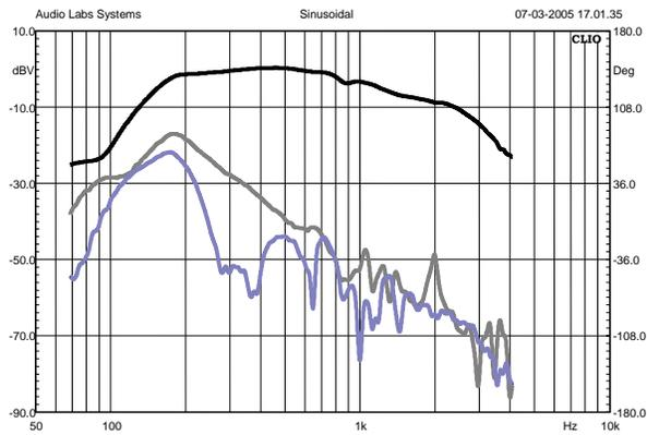
Figure 41: 600-type **with AIC**, driving current response & distortion
