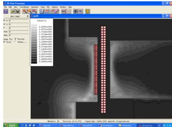
Figure 26: 500-type 2 kHz with AIC, shot 1 - J [A/m<sup>2</sup>]
