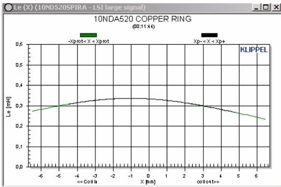
Figure 54: Le vs. displacement in a 500-type speaker with the ring in the gap
