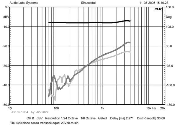
Figure 42: **Standard** 500-type, driving current response & distortion
