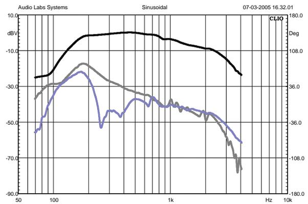
Figure 40: **Standard** 600-type, driving current response & distortion
