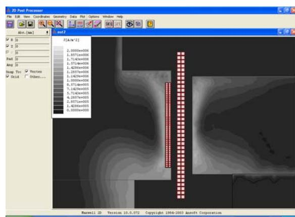
Figure 16: 500-type 250Hz with AIC, shot 3 - J [A/m<sup>2</sup>]
