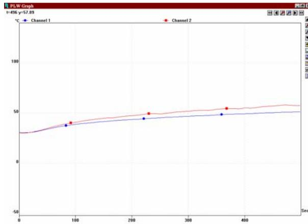
Figure 57: Difference in temperature after about 8 minutes at  $\frac{1}{4}$  of power between the AIC-equipped speaker (the upper curve) and the same speaker but equipped with a copper shorting ring in the gap (lower curve).
