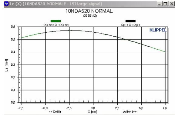
Figure 52:  $L_e$  vs. displacement in the **standard 500-type**
