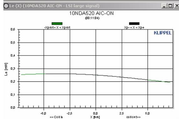
Figure 55: Le vs. displacement in a 500-type speaker with AIC connected
