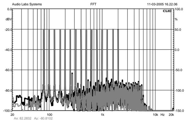
Figure 48: driving current FFT multi-tone test over a 500-type with a ring under the pole piece (gray) and without it (black).
