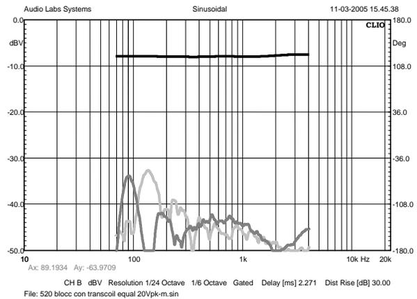
Figure 43: 500-type **with AIC**, driving current response & distortion
