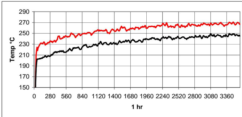
Fig 6 – First hour results of the same AES standard power test (temperature versus time, 15 inch speaker comparison); black plot ISV, red plot external coil.
