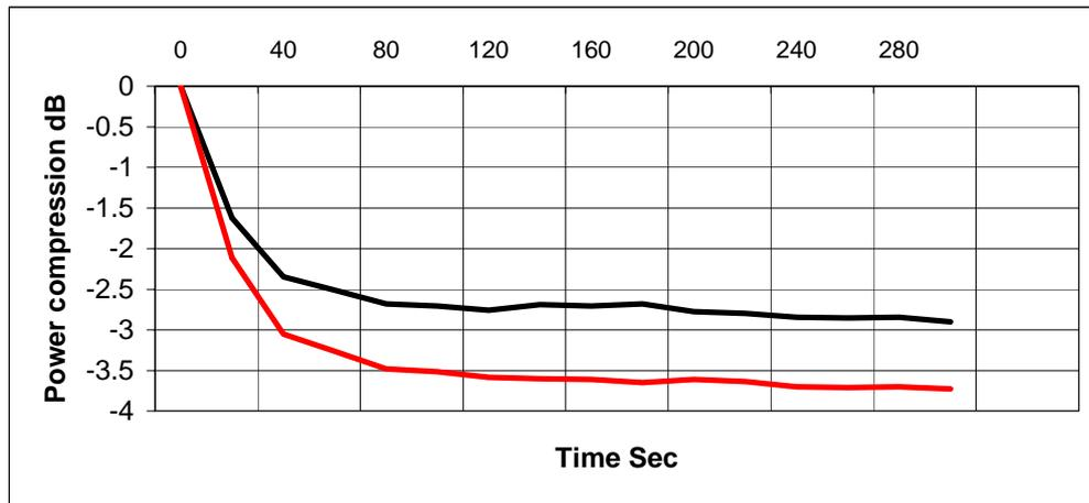
Fig 7 – Power compression in the first 5 minutes of an AES standard power test (temperature versus time, 15 inch speaker comparison): black plot ISV, red plot external coil.
