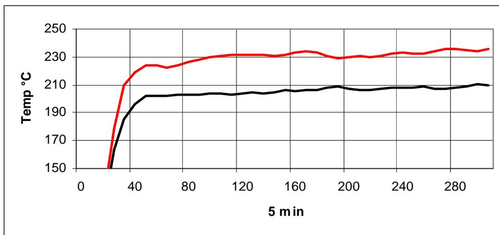
Fig 5 – First 5 minutes of an AES standard power test (temperature versus time). 15 inch speaker comparison, black plot ISV voice coil, red plot conventional external type. The 25°C difference is mainly due to increased conduction surface (Fig 1 vs. Fig 3).
