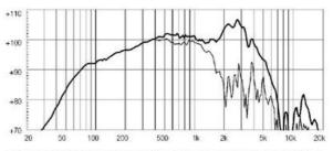
FREQUENCY RESPONSE CURVE OF 12MB700 MADE ON 50 LIT. ENCLOSURE TUNED 60HZ IN FREE FIELD (4PI) ENVIRONMENT. ENCLOSURE CLOSES THE REAR OF THE DRIVER. THE THIN LINE REPRESENTS 45 DEG. OFF AXIS FREQUENCY RESPONSE
